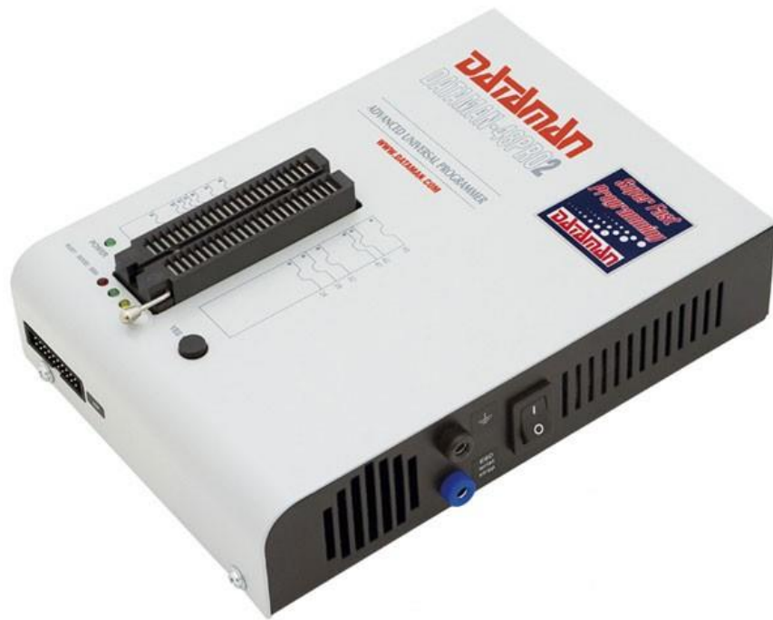
Slika 4.11 Dataman 48Pro2 Super Fast Universal ISP Programmer 23
