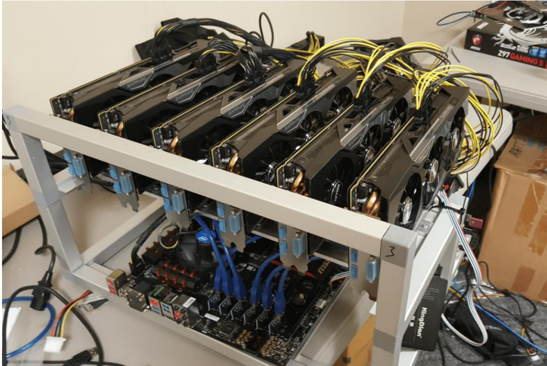
Slika 2.5 Konfiguracija za rudarenje (mining rig). Izvor: https://blockoperations.com/build-6-gpu-zcash-headless-mining-rig-ubuntu-16-04-using-claymore/ (25.07.2018. u 20:15)
