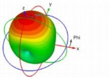
(b) Patch Antenna 3D Radiation Pattern
