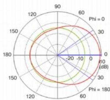
(c) Patch Antenna Azimuth Plane Pattern
